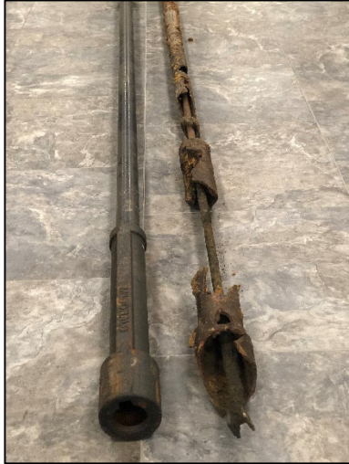
Comparison of new curb box (left) to curb box from 2023 project (right)
